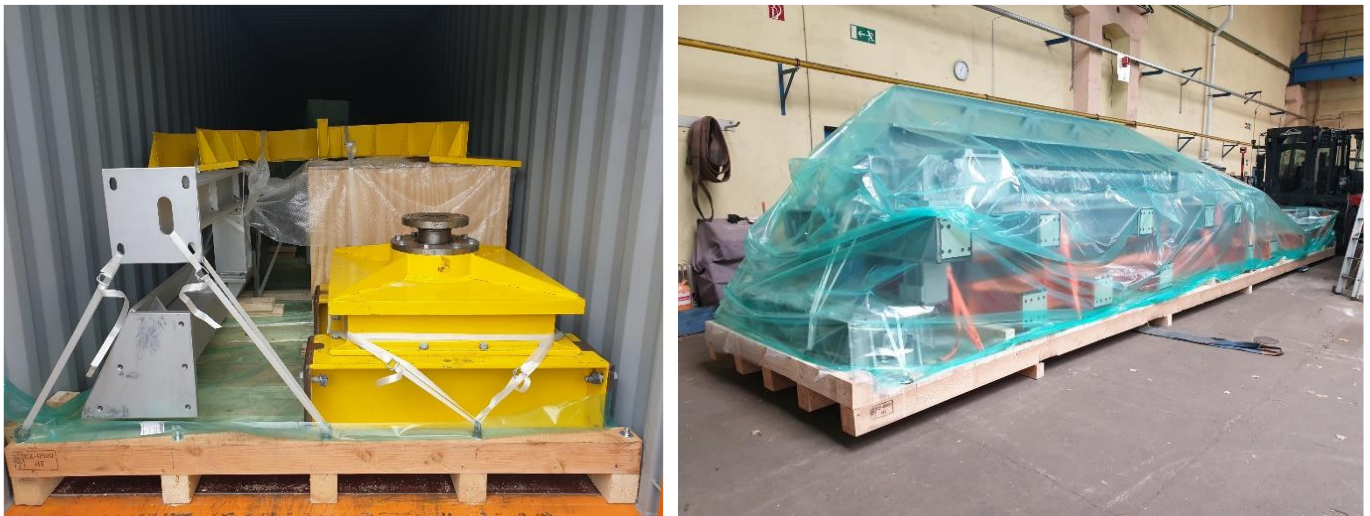
Fig. 3.1.1-1 packed machine components inside container (left) / on wooden crate (right)
