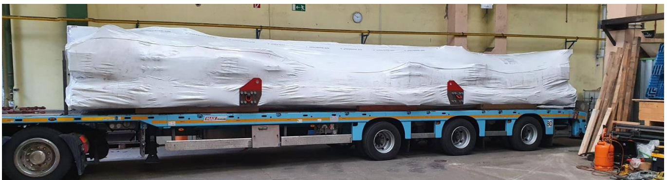
Fig. 3.1.1-2 oversized package on a truck (red lashes are for lifting and securing)
